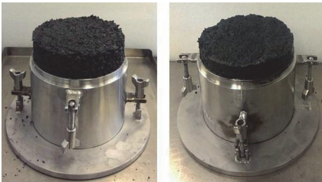
Figure 1.5.7 Photographs showing valid tests for a partially saturated test portion (left) and a near fully saturated test portion (right)
