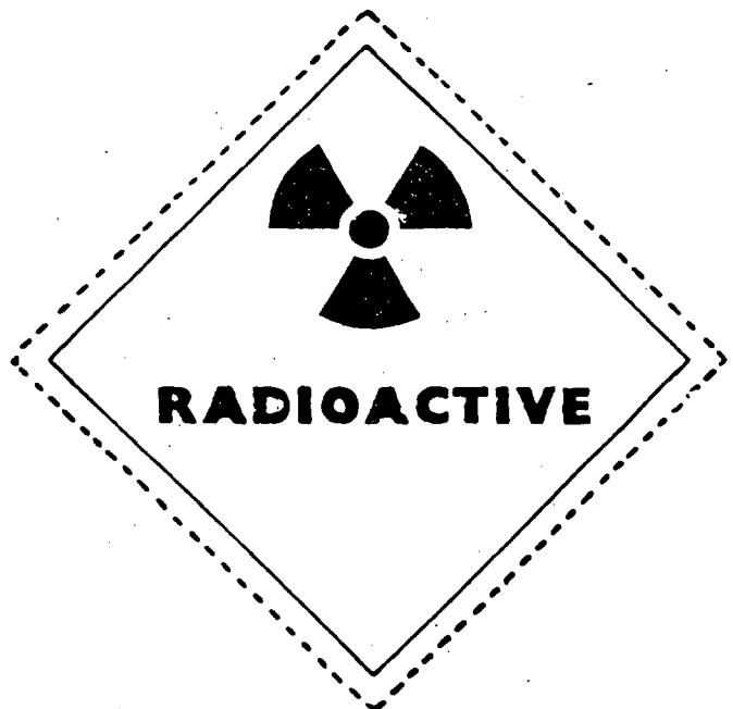
(Minimum length of side: 15 cm) Symbol and inscription black on white ground
